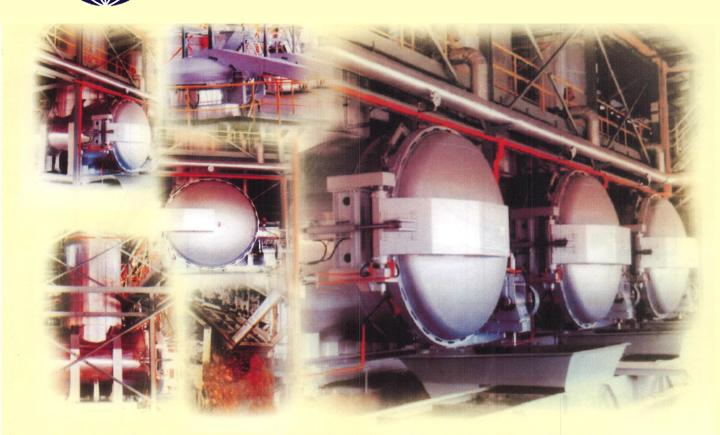
UVE Automated Steriliser X25 (UVEAS) System was developed to simplify the whole sterilisation station to produce the finest and most consistent ffb sterilisation effortlessly and unobtrusively. FFB is conveyed via scraper conveyor from the loading ramp to the UVEAS. After sterilisation, the sterilised bunch is conveyed via scraper conveyor to the thresher.
